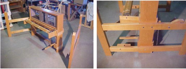
Step 2: Put the treadles on. There are pins on the back side of the lower front legs to align the treadle bar. Make sure the back of the treadles are on top of the treadle rest. Because of the brake treadle the treadles can only go on one way. Secure them with the 1/4" nut and washer. Once you have the treadles on, hook up the chain in the back for the brake release.
