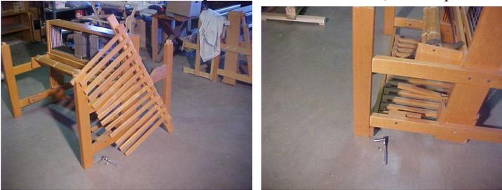
Step 3: Put the warp beam on. Secure with the rivet pins.
