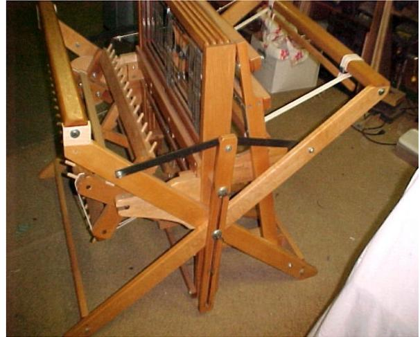
**COMPACT series loom:** These looms were designed to have the Warp Beam taken off and the arms that hold it swing down. The cross beam above it (Top Back Bar) is on arms that swing up. Doing these things allows the loom to pass through a standard (3') doorway.
