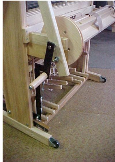
GEM II with friction brake and single wheels on bottom leg rail.
