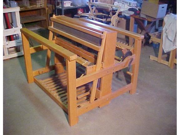
**X FRAME series loom:** The X Frame looms were made to fold when moved or not in use. They are easy to identify because the side leg assembly makes an "X". The Warp Beam is attached to a permanent arm.
